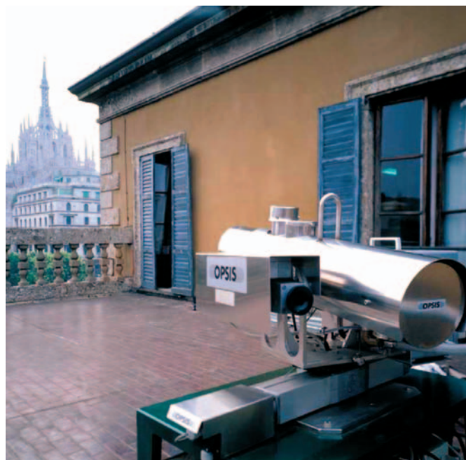
ABOVE: An Opsis Open Path Air Quality Monitoring Station installed on a rooftop in Milan, Italy
